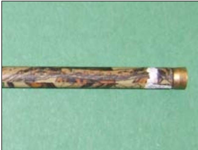
This is the shaft the aluminum ferruled Outback show above was mounted on. Note area of shaft finish removed by the bone. The arrow stopped in the rib. A broadhead's ability to relieve bone pressure against broadhead and shaft is an important penetration feature, as is total arrow integrity!
