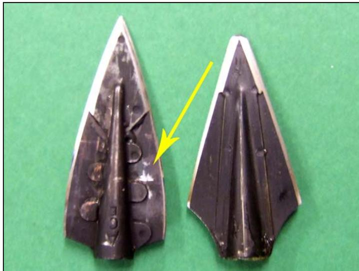
The Ace Standard (L) and Magnus II. Note the abraded area just forward of one of the Ace's ferrule-lugs (arrow). These appeared several time on the Ace broadheads, and are areas where bone has gouged into the metal, as the lugs forced their way through the bone.
