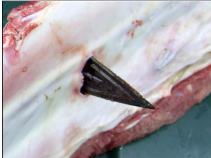
**This was all the rib-penetration the Ace Super Express could muster. The wide-cut and surface lugs attaching the ferrule cause high penetration-resistance.**
