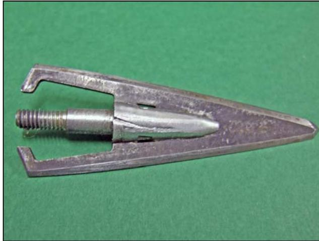
The aluminum ferrule on this double-bevel Outback Supreme shows a deep gouge inflicted by a buffalo rib. A number of similarly damaged aluminum ferrules were recorded during their testing.
