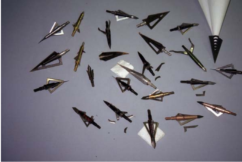
Some of the broadheads damaged during 2004 testing.
