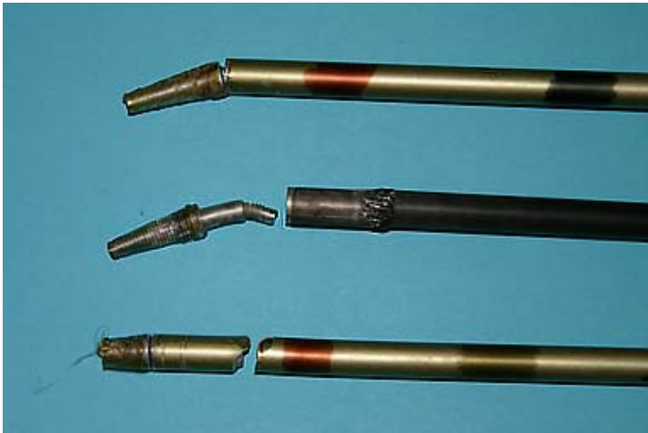
Aluminum adaptors/inserts are a decidedly weak point in the synthetic shaft arrow system.
