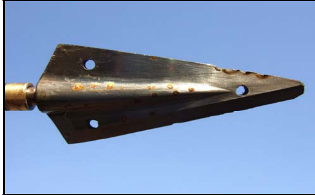
Second set of edge chips on the one, likely over-hardened, prototype Ashby broadhead.
